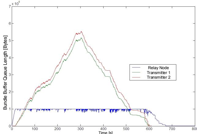
Fig. 5. Bundle Buffer Queue Length in case of 1 Mbytes buffer capacity (only relay node) and propagation delay 5 s.
