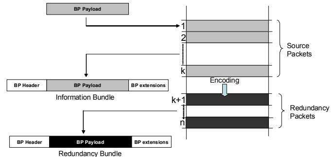
Fig. 1. The encoding scheme within the Bundle Protocol (BP) entity.
