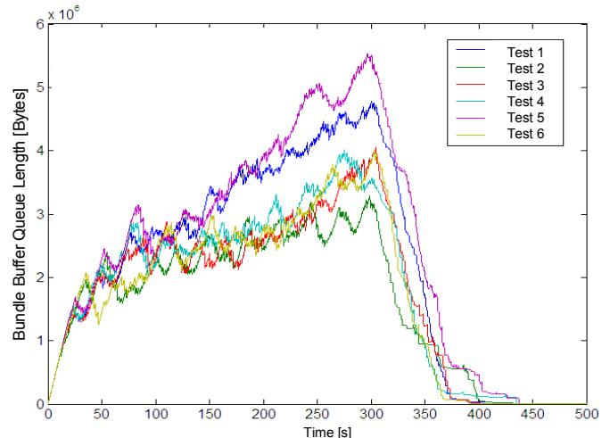
Fig. 3. Bundle Buffer Queue Length in case of unlimited buffer capacity and propagation delay 5 s, for several realisations (Tests 1 through 6).
